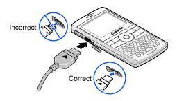
Plug the adaptor into a standard AC wall outlet. When charging is finished, unplug the adaptor from the power outlet.
